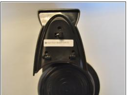
Remove and set aside the three 1.3 mm Philips #2 screws holding the plastic cover in place.
