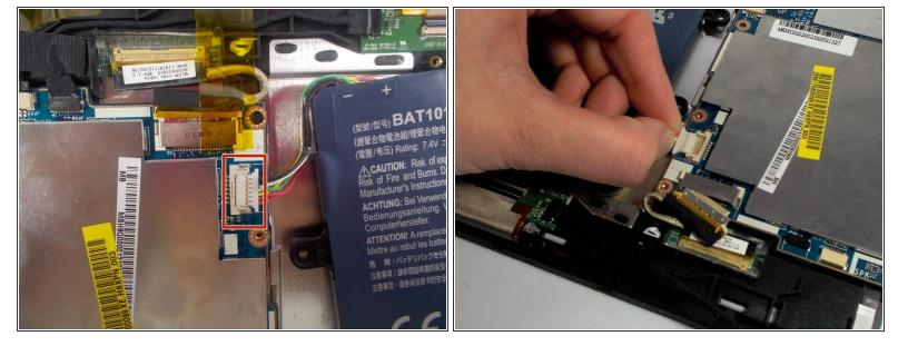
Lift the battery out of the device, and disconnect the cable attached to the motherboard by pulling it out to the side not lifting it up.
