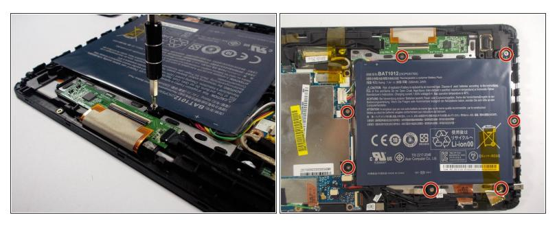
Using a Phillips #00 screwdriver remove the 4.0 mm screws holding the battery in place.
