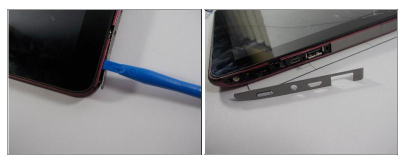
With the plastic opening tool pry open the grey plastic siding on both sides of the tablet.
