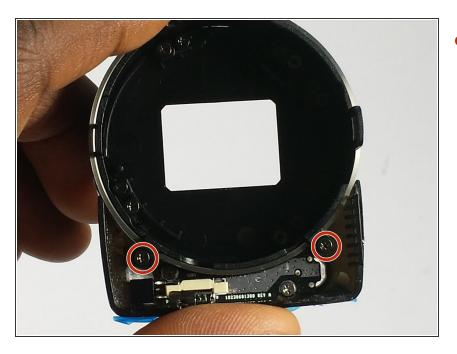
• Take out the two 20 mm screws that attach it to the shutter.
