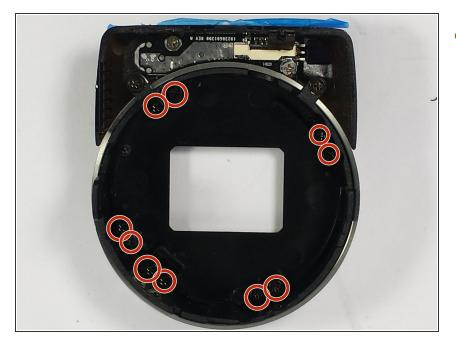
Remove the ten 30 mm Phillips #0 screws from the front lens.
