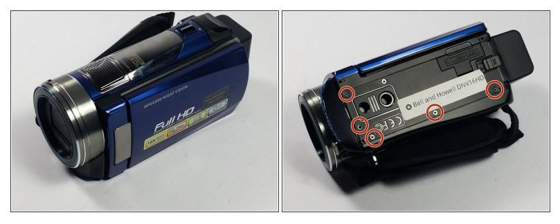
• Remove the five 30mm Phillips #0 screws on the bottom of the camera.
