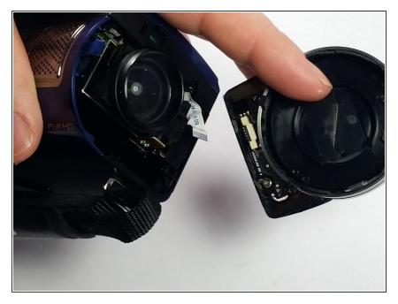
It will still be connected by a plastic film. This can also be disconnected by pulling up the white part where it connects to the light circuit board.
