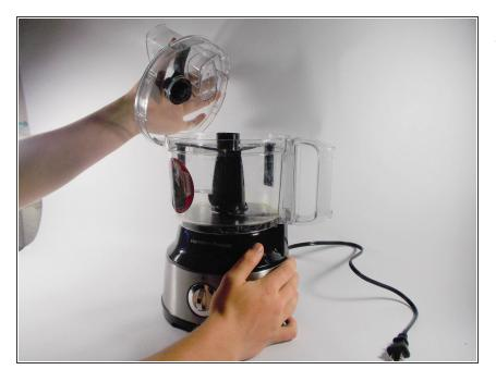
• Unscrew the cover by turning it counterclockwise.
