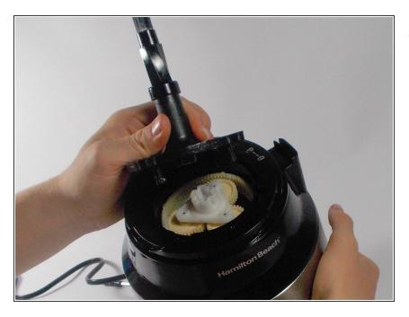
• Lift the driveshaft off of the base.
