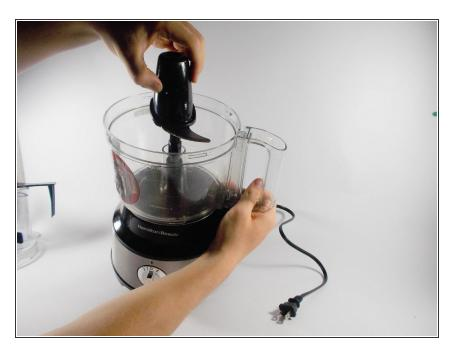
Gently lift the blade mechanism from the top black piece.
