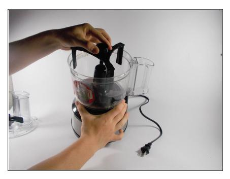
Lift the bowl scraping mechanism up and out of the bowl.
