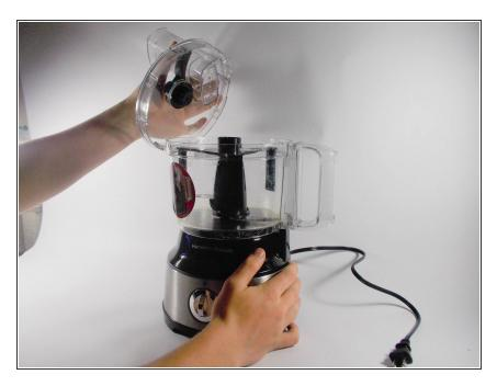
Unscrew the cover by turning it counterclockwise.
