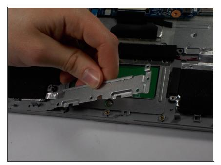
Lift and remove the metal bracket from below the touch pad.
