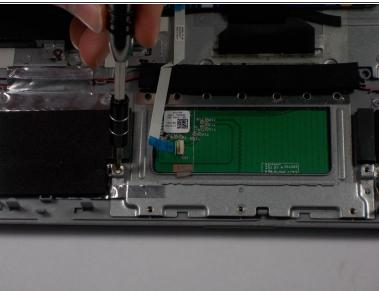
Remove the three visible screws below the touch pad that hold the bracket in place.
