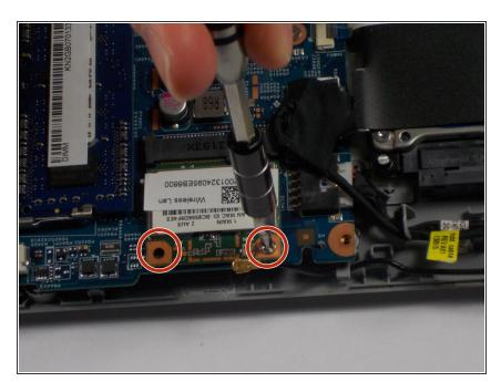
Unscrew the two 3mm screws holding the network card in place.
