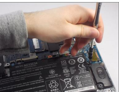
Carefully unscrew the two 5mm screws holding the battery in place.
