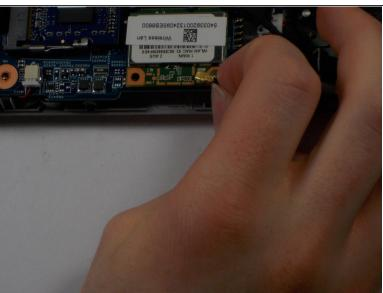
Start by removing the antenna cable attached to the network card.
