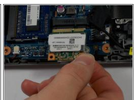
Carefully remove the network card by pulling it backwards, out of the slot that it is plugged into.
