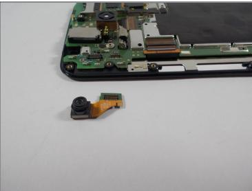
• Use the flat end of the nylon spudger to gently pry up on the front camera connector.
