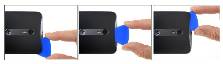
Slice through the adhesive along the top edge of the phone, pulling the pick out slightly to guide it around the rear-facing camera.
