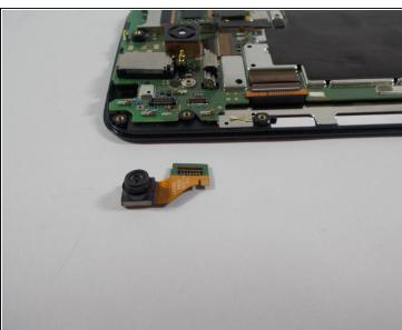
• Use the flat end of the nylon spudger to gently pry up on the front camera connector.
