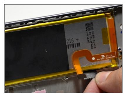
Locate adhesive strip underneath the battery and grip with your thumb and forefinger. Slowly pull on the adhesive strip until it's off to release adhesive securing battery.
