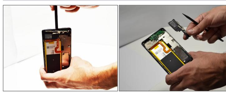
• **Gently**, use the flat end of the <u>Spudger tool</u>, or a metal opening tool to **lift** and **remove** the loudspeaker from the phone. The loudspeaker is the entire portion of the phone where the screws were extracted.
