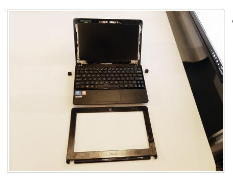
When the screen case has been successfully removed, the laptop should resemble the photo shown here.
