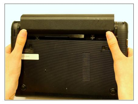
Push the battery upwards and out of the laptop as shown.
