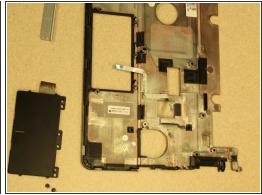
• Detach the tape connecting the trackpad to the trackpad base, and carefully remove the trackpad.
