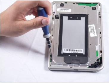
• Using the T5 Torx screwdriver, remove the ten T5 screws from around the edges of the silver midframe.
