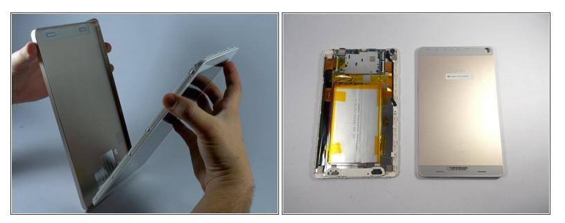
• Using your hands and the separating tool, remove the back cover from the device.
