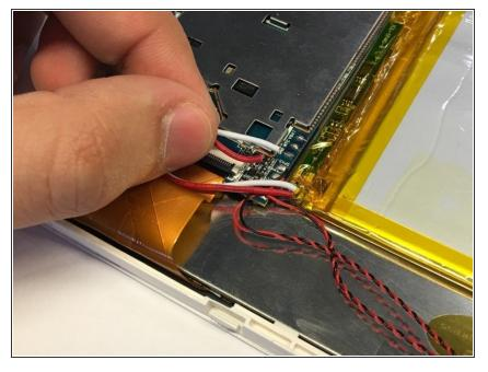
• The red and white wires connecting the battery to the motherboard must be desoldered. Refer to the <u>Soldering Technique Guide</u> for instructions on how to do this. (Be sure to desolder the wires from the battery AND the motherboard.)
