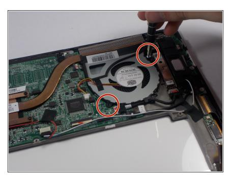
Remove two 3.0mm Phillips J0 screws using a Phillips screw driver.
