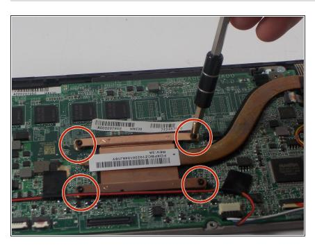
Remove four 3.5mm Phillips J0 screws from the heat sink.
