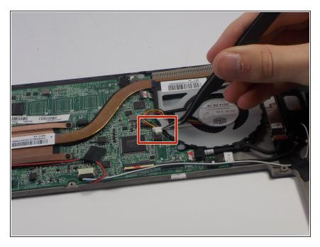
Remove the power connector from the fan using a pair of tweezers.
