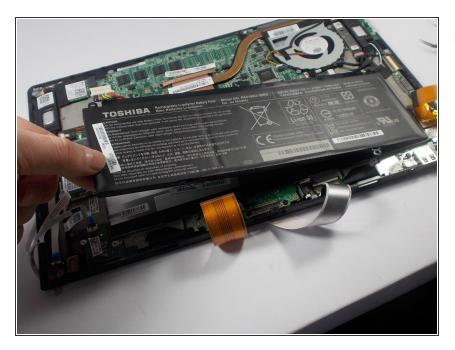
Remove the battery from its holding position.
