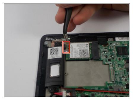
• Remove the black and white cables attached using ESD safe tweezers.
