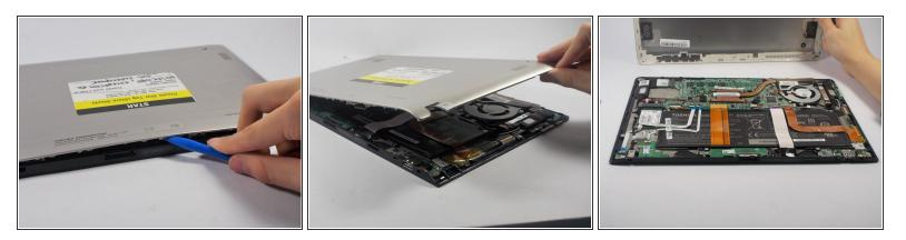
Remove the base of the tablet from the screen using a plastic opening tool.
