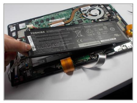
• Remove the battery from its holding position.
