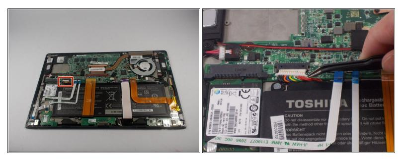
• Remove the battery power connector using ESD safe tweezers.
