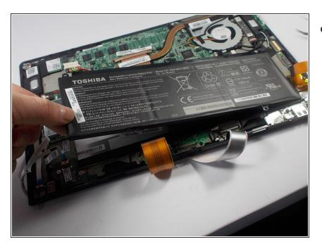
Remove the battery from its holding position.
