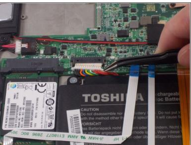
Remove the battery power connector using ESD safe tweezers.
