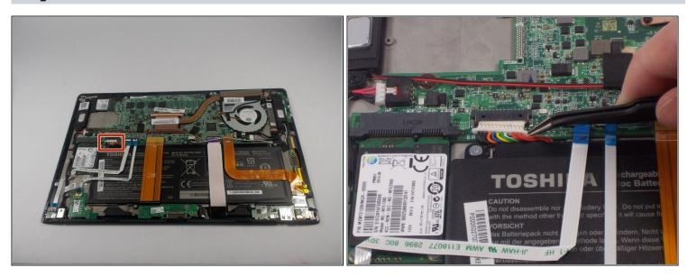
Remove the battery power connector using ESD safe tweezers.
