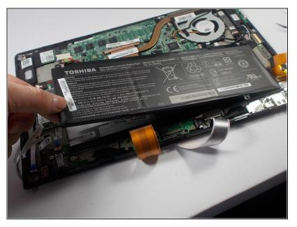
Remove the battery from its holding position.
