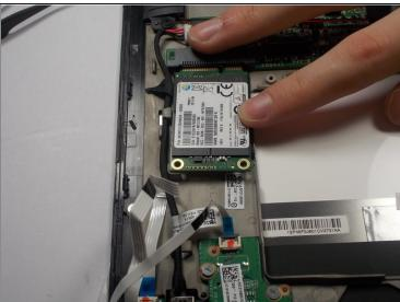
Remove the two screws using a J0 Phillips screw driver
