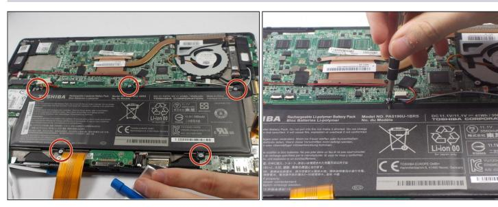
• Remove five 3.5mm Phillips J0 screws using a Phillips screw driver.
