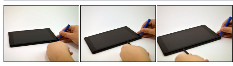
• Slide a plastic opening tool and spudger along the underside of the screen using enough force to peel the screen and the adhesive strip from the other half of the device.
