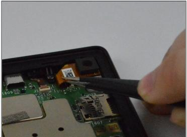
• Pop the camera out of the rear-facing camera casing by carefully pulling the orange cable with the tweezers.
