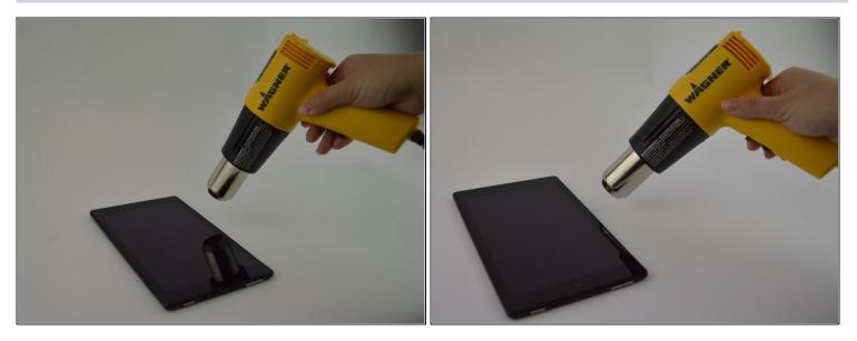
• Heat the edges of the screen with a heat gun on the lowest setting by using sweeping motions from about 8-10 inches away.
