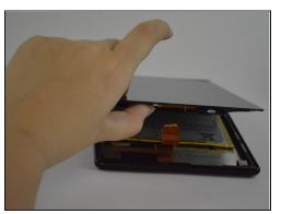
• To remove the screen from the device, use tweezers to gently pull the orange cable from its connection to the screen.
