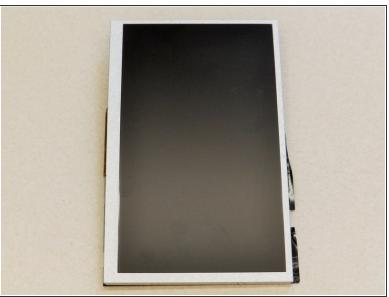
• The digitizer is now free from the front frame and ready to be repaired or replaced.
