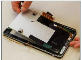
Use a plastic opening tool to wedge underneath the digitizer and pry up, lifting the digitizer out of the frame.
