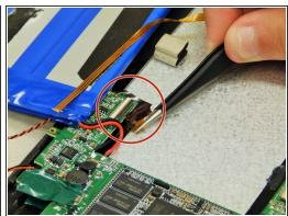
Carefully remove the remaining ribbon cables using the tweezers. Make sure that all ribbon cables are detatched before attempting to remove the motherboard.
