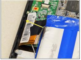
Locate the black tape connected to the battery and peel it back as indicated in the images.
