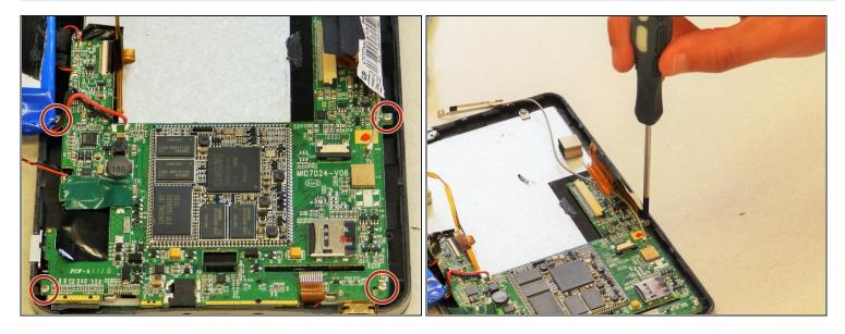
• Locate the four 5mm screws holding the motherboard in place and remove them using the Phillips #0 Screwdriver.
