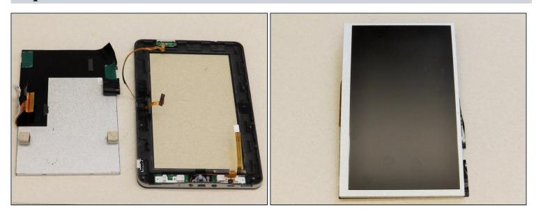
• The digitizer is now free from the front frame and ready to be repaired or replaced.
