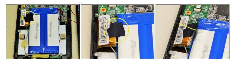
Locate the black tape connected to the battery and peel it back as indicated in the images.
