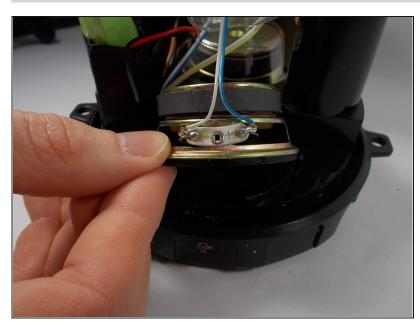
• Lift the horn from its fitting by pulling it. Position it in a manner that is easy to work with.
