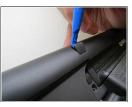
Locate the four rubber grips on the bottom of the speaker. Use the plastic opening tool to remove the grips, exposing the underlying screws.
