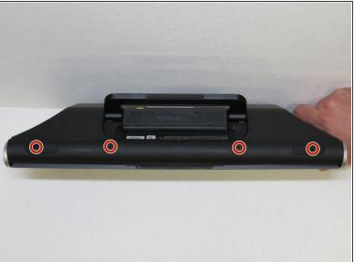
Using a Phillips #1 screwdriver, remove the four 5mm screws that were underneath the four rubber grips.
