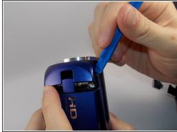
Use the plastic opening tool to loosen the plastic case of the camcorder.
