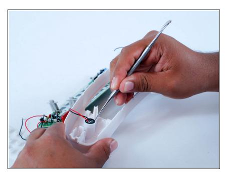
Use metal spudger to remove the microphone
