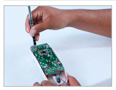
Remove the two 10 mm screws using the 1/4" driver and a J1
