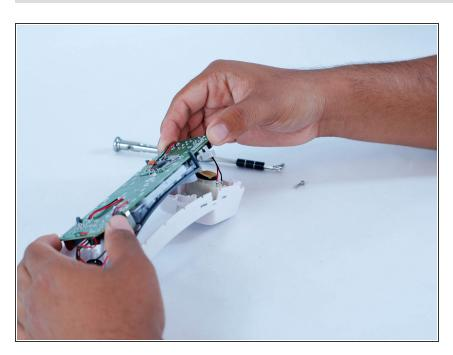
Carefully move the motherboard up to remove it.
