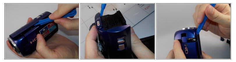
• Use the plastic opening tool to loosen the plastic case of the camcorder.
