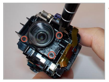
Remove the 3 (4mm) screws on the front of the lens using the Philips #0 Screwdriver.
