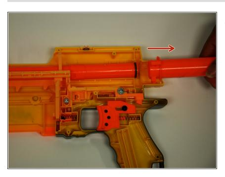
Pull plunger away in the same motion as in step 7 with the plunger lock.
