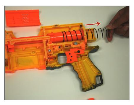
Now remove the main firing spring from the rear of the device by gently pulling it.
