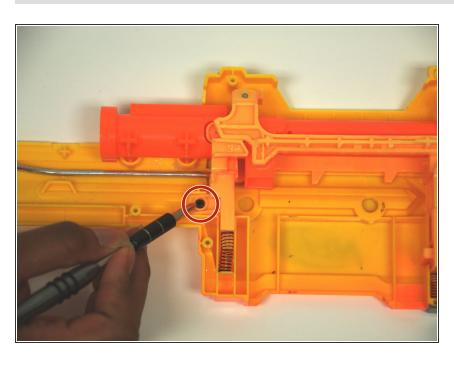
Remove the 5 mm Phillips #0 screw holding in the chamber lock mechanism.
