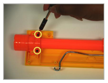
Remove the two 5 mm Phillips #0 screws holding the muzzle in place.
