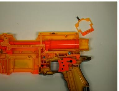
Push the barrel forward and remove the square piece that holds the back of the barrel in place.
