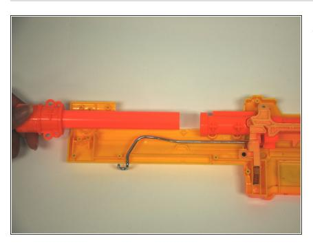
Remove the barrel and muzzle assembly from the gun body.
