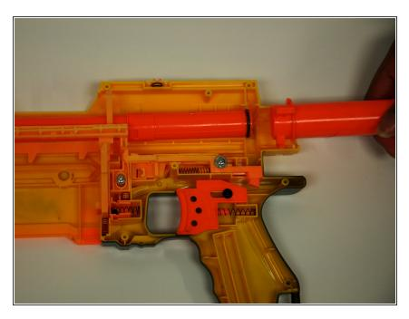
Pull the air cylinder and plunger assembly out of the rifle.
