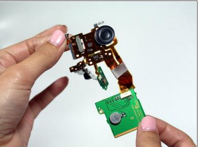
Carefully pull the speaker out of the casing.
