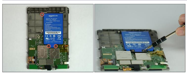
• Unscrew the three 3.0 mm Phillips #000 screws that are securing the battery.
