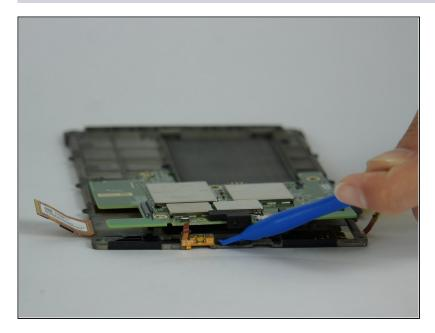
• Use a plastic opening tool to lift the motherboard upwards from the frame.
