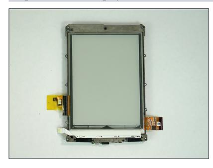
The touchscreen is attached to the rest of the frame.
