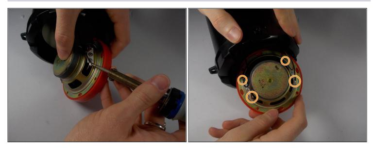
• To remove the the wires from the subwoofer terminals, use a soldering iron to reheat the solder at each of the four points of connection.
