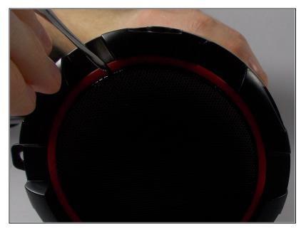
• Use a metal spudger to remove the mesh speaker cover by wedging the narrow end into the center of the outer edge of the mesh touching the red plate.
