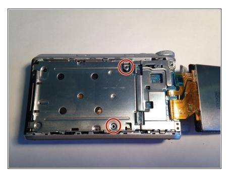
Remove two more 3.2 mm screws on the silver panel using your Phillips #000 Screwdriver.
