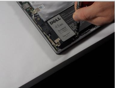
Locate the battery at the bottom of the computer and remove the four 3mm screws with a Phillips #0 head that hold the battery down.
