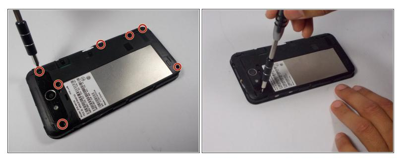
Remove the seven 3.175mm Phillips head screws from the inner back located at the top, uppermiddle-right, middle-right, lower-right, and bottom.
