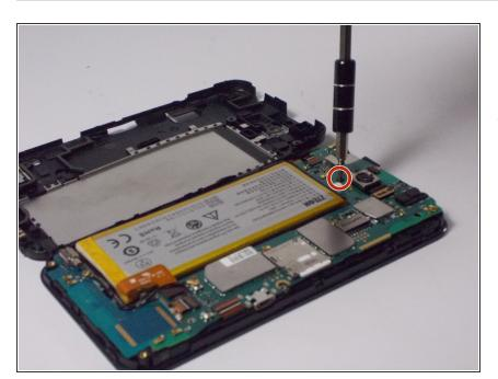
Remove the one 2.381mm Phillips head screw from the motherboard located in the upper-middle part of the phone next to the bottom left corner of the back camera.
