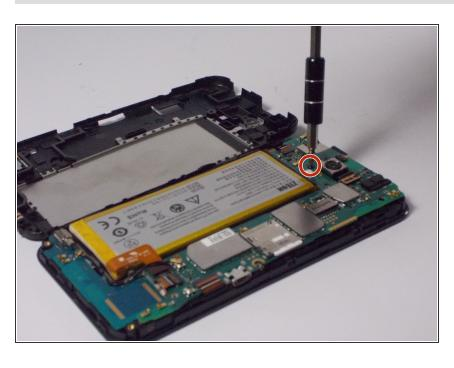
Remove the one 2.381mm Phillips head screw from the motherboard located in the upper-middle part of the phone next to the bottom left corner of the back camera.
