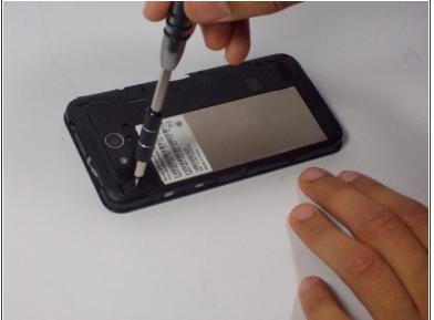
Remove the seven 3.175mm Phillips head screws from the inner back located at the top, upper-middle-right, middle-right, lower-right, and bottom.
