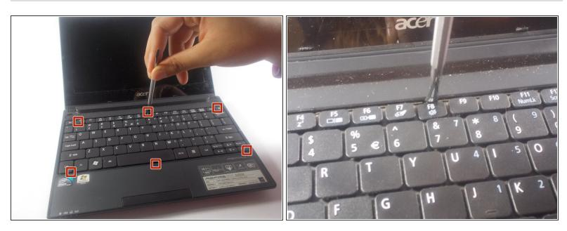
Using plastic opening tools press down the 6 clips located around the keyboard.
