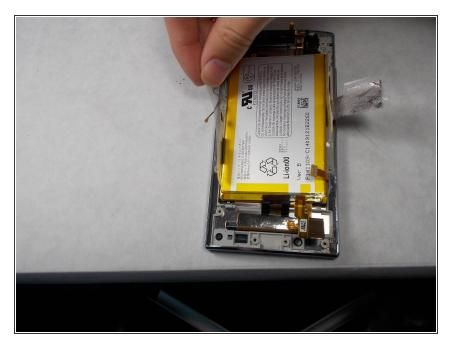
• Peel off the tape holding the battery down.
