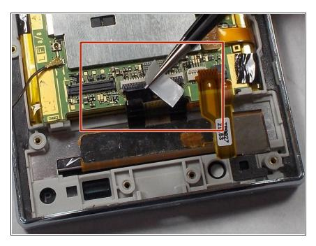
Use the tip of a spudger or your fingernail to flip up the small retaining flap. Then pull the cable out using tweezers.
