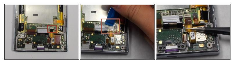
• To disconnect the cable, use the tip of a spudger or your fingernail to flip up the small retaining flap. Then, you can safely pull the ribbon cable out.
