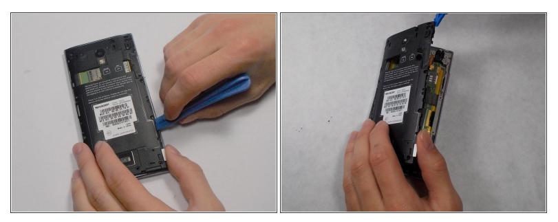
Pry open the back panel using a plastic opening tool. Do this around the edges until you are able to lift it off.
