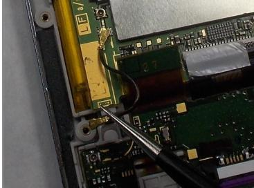
• Remove the wire from the two marked connections using tweezers to pull the wire apart from the device.
