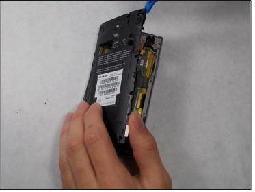
• Pry open the back panel using a plastic opening tool. Do this around the edges until you are able to lift it off.
