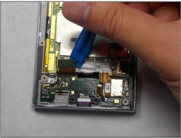
Disconnect the wire by lifting it up with a plastic opening tool.
