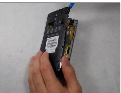
Pry open the back panel using a plastic opening tool. Do this around the edges until you are able to lift it off.
