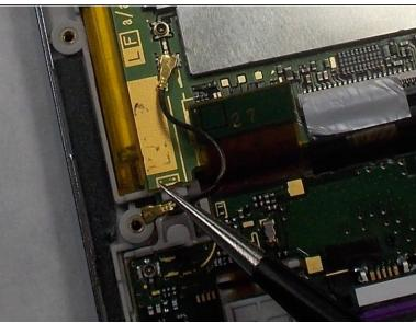
Remove the wire from the two marked connections using tweezers to pull the wire apart from the device.
