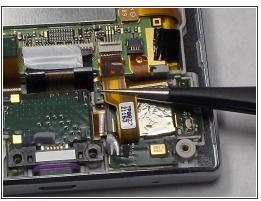
To disconnect the cable, use the tip of a spudger or your fingernail to flip up the small retaining flap. Then, you can safely pull the ribbon cable out.
