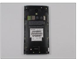
Peel back the back cover of the phone from the access point to remove it. It should come off easily using your hands.
