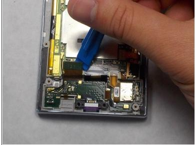
Disconnect the wire by lifting it up with a plastic opening tool.
