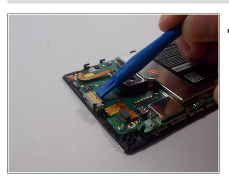
Remove USB port cover using the plastic opening tool, or your hand. It can be removed easily.
