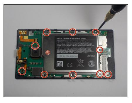
Remove all 10 T5 screws on the motherboard. All screws are 4.5 mm Torx T5 screws.
