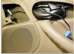
Detach the wires on the handle housing with a flathead screwdriver by pushing upwards on the release slot.
