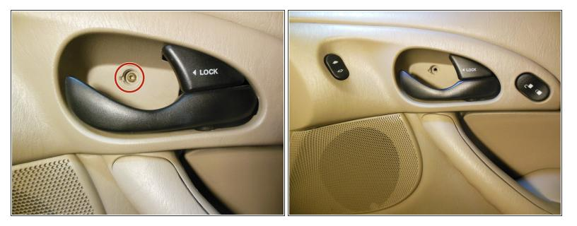
Remove the screw that is holding the handle housing with a T20 Torx screwdriver.
