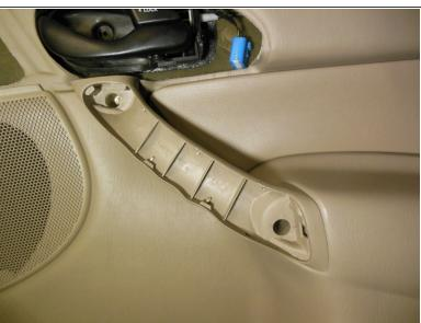
Remove the cover on the door grip by prying gently with a flathead screwdriver.
