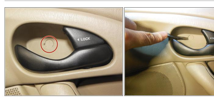
Remove the screw cover in the handle housing using a flathead screwdriver.
