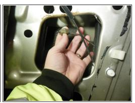
• Detach the door latch rod from the handle bracket by pulling the plastic end out of the metal loop.
