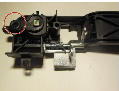
• Pull the locking rod free from the handle bracket and remove the broken handle bracket.
