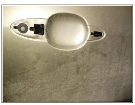
Remove the outside door handle by prying gently with a flathead screwdriver to loosen, and then slide it back.
