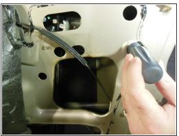
Remove the two screws holding the handle bracket with a T20 Torx screwdriver.
