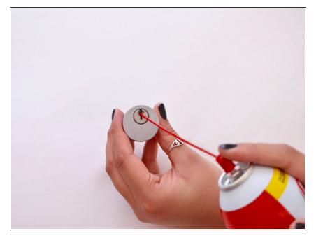
• Spray GumOut parts cleaner into the key cylinder to lubricate chamber.
