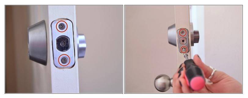
• Use a Phillips screwdriver to remove both of the <sup>3</sup>/<sub>4</sub>-inch screws from the strike plate.
