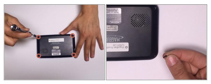
Remove all four 5mm screws from the back of the device using a Phillips Head screwdriver size 000.
