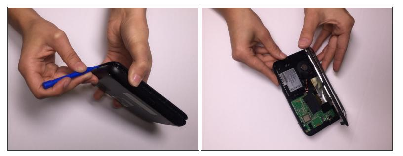
• Open the casing of the device using a plastic spudger.
