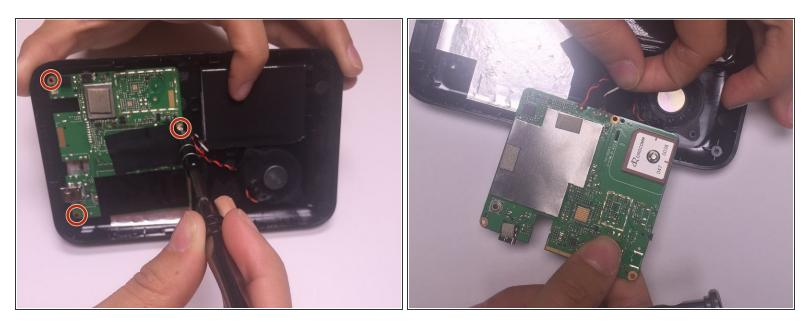
Remove the motherboard from the device by unscrewing all three 4mm screws that are connecting it to the casing with a Phillips Head screwdriver size 000.
