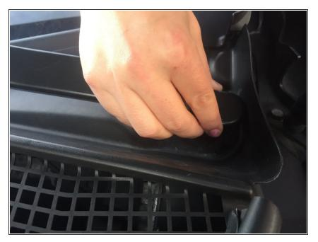
Place the bolt cover back over the bolt and push it down into clipped position.
