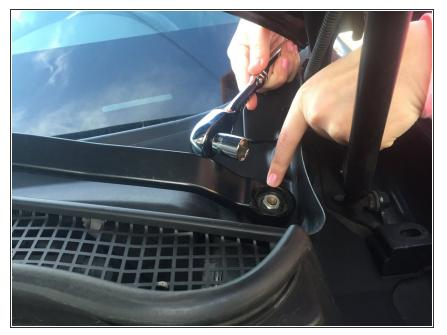
• After removing the bolt cover, you will find the bolt that holds the wiper arm onto the vehicle.
