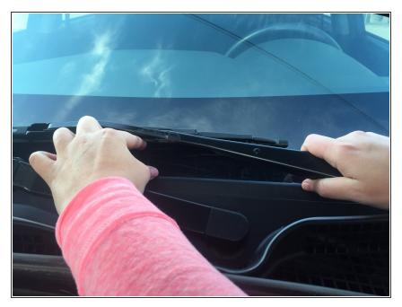
• There should be approximately 2 inches of space between the bottom of the windshield and the wiper in proper resting position.
