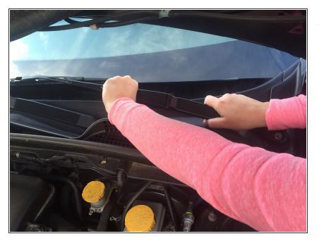
Adjust the windshield wiper arm such that it is in the proper resting position.
