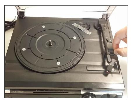
• Next, lift up the clip that holds the tone arm in place and lift the tone arm out.
