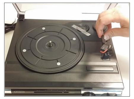
• The cartridge and needle is the red piece at the end of the tone arm. To remove it, simply grab the end on each side and pull back slowly. The piece should slide right off the tone arm
