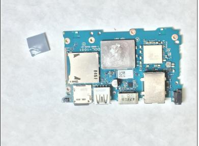
Remove the old thermal pad with an ESD safe tool, like a Jimmy.
