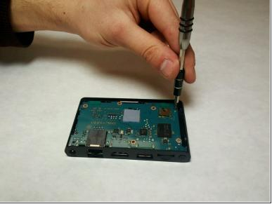
Remove the last 6mm Phillips #0 screw from the motherboard.
