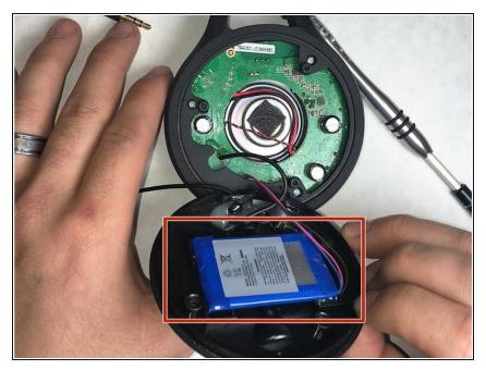
The battery is adhered to the back cover of the JBL Clip Plus, slowly lift the battery away from the case, using a spudger to pry the battery away from the adhesive.
