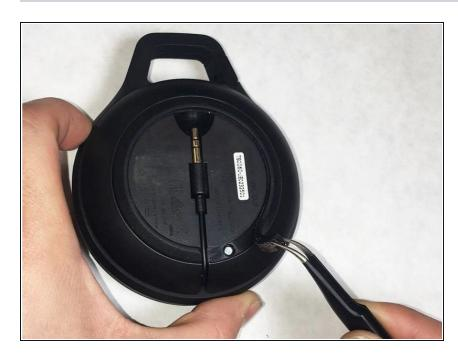
Use the angled tweezers to carefully pull the rubber bumper off the back side of the device
