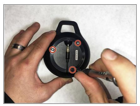
There will be three 6mm philips head screws under that rubber bumper, remove these three screws.
