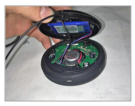
The back cover should lift open easily and the components should be visible.
