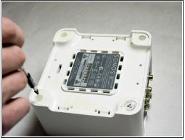
• Remove the four 7.5mm length Philips head screws under the rubber cover.
