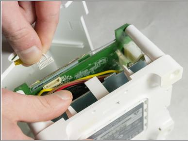
• Remove the connection for the front buttons to fully remove the cover.
