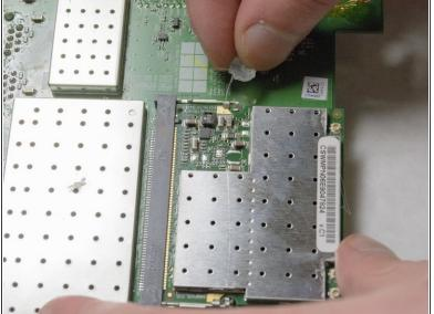
Remove the two pieces of glue holding the WIFI card in place.
