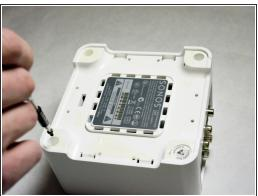
• Remove the four 7.5mm length Philips head screws under the rubber cover.
